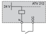
“PLC” position with PLC transistor outputs
